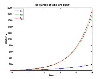
**Evaluating the Solution.** The method implemented in dde23 produces a continuous solution over the whole interval of integration  $[t_0, t_f]$ . You can evaluate the approximate solution, S(t), at any point in  $[t_0, t_f]$  using the helper function deval and the structure sol returned by dde23.
