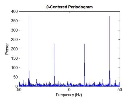
The rearrangement makes use of the periodicity in the definition of the DFT (see "Discrete Fourier Transform (DFT)" on page 9-2).
