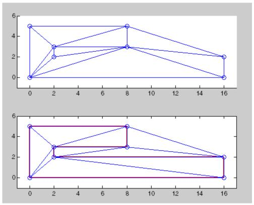
The top plot show the original unconstrained Delaunay triangulation. The bottom plot shows the triangulation subject to the constraints C. The inOutStatus method of DelaunayTri returns the in/out status of the triangles in a 2-D constrained Delaunay.
