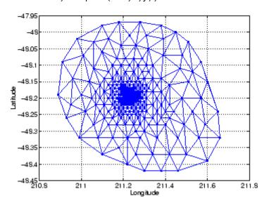
Mesh and Surface Plots. Add the depth data (z) from seamount, to the Delaunay triangulation, and use trimesh to produce a mesh in three-dimensional space. Similarly, you can use trisurf to produce a surface:
