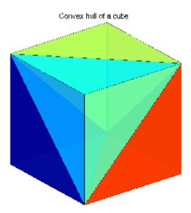
**Delaunay Tessellations.** A Delaunay tessellation is a set of simplices with the property that, for each simplex, the unique sphere circumscribed about the simplex contains no data points. In two-dimensional space, a simplex is a triangle. In three-dimensional space, a simplex is a tetrahedron.
