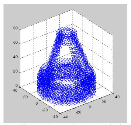
The variable  $\mbox{tet}$  is a triangulation of X. You can plot it directly with the function  $\mbox{tetramesh}.$
