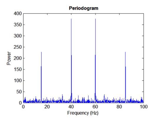
The first half of the frequency range (from 0 to the Nyquist frequency fs/2) is sufficient to identify the component frequencies in the data, since the second half is just a reflection of the first half.
