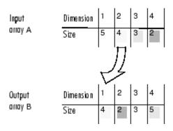
The order of dimensions in permute's argument list determines the size and shape of the output array. In this example, the second dimension moves to the first position. Because the second dimension of the original array had size 4, the output array's first dimension also has size 4.
