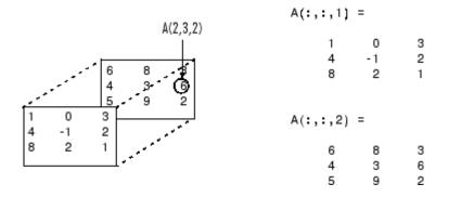
As you add dimensions to an array, you also add subscripts. A four-dimensional array, for example, has four subscripts. The first two
