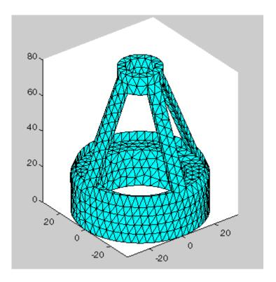
You can also create a triangulation in MATLAB with the DelaunayTri constructor and query it with TriRep methods. DelaunayTri creates Delaunay triangulations and related constructs from a set of points in 2- and 3-D space.
