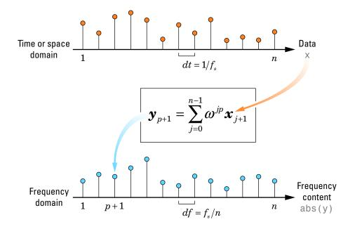
The first element of y, corresponding to zero frequency, is the sum of the data in x. This DC component is often removed from y so that it does not obscure the positive frequency content of the data.
