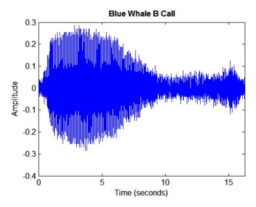
Use fft to compute the DFT of the signal. Correct the frequency range for the factor of 10 speed-up in the data:
