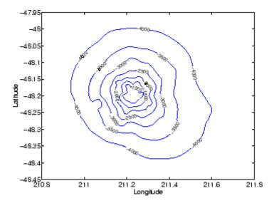
The arguments for meshgrid encompass the largest and smallest x and y values in the original seamount data. To obtain these values, use min(x), max(x), min(y), and max(y).
