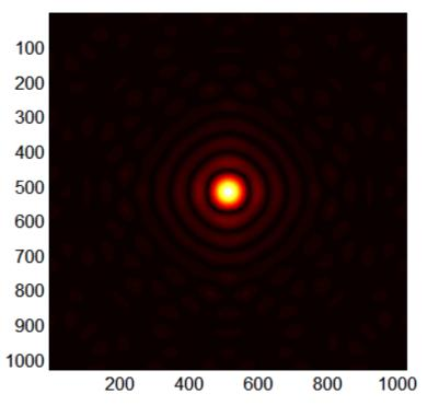
The logarithm helps to bring out details of the DFT in regions where the amplitude is small:
