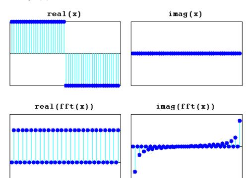
The midpoint of the DFT (or the point just to the right of the midpoint if the length is even), corresponding to half the sampling frequency of the data, is the *Nyquist point*. For real x, the real part of the DFT is symmetric about the Nyquist point, and the imaginary part is antisymmetric about the Nyquist point.
