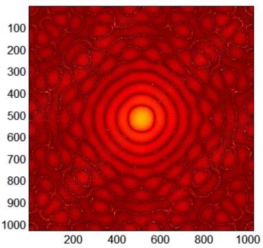
Very small amplitudes are affected by numerical round-off. The lack of radial symmetry is an artifact of the rectangular arrangement of data.
