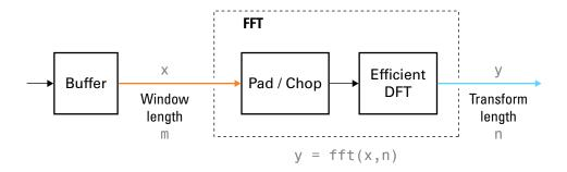
The execution time of an FFT algorithm depends on the transform length. It is fastest when the transform length is a power of two, and almost as fast when the transform length has only small prime factors. It is typically slower for transform lengths that are prime or have large prime factors. Time differences, however, are reduced to insignificance by modern FFT algorithms such as those used in MATLAB. Adjusting the transform length for efficiency is usually unnecessary in practice.
