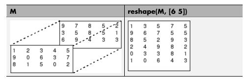
The reshape function operates in a columnwise manner. It creates the reshaped matrix by taking consecutive elements down each column of the original data construct.
