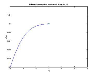
**5** Use continuation to solve the problem and plot subsequent solutions. The example then solves the problem for infinity = 4, 5, 6. It uses bypinit to extrapolate the solution sol for one value of infinity as an initial guess for the next value of infinity. For each iteration, the example prints the computed value of f''(0) and superimposes a plot of the solution in the existing figure.
