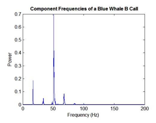
The B call is composed of a fundamental frequency around 17 Hz and a sequence of harmonics, with the second harmonic emphasized.
