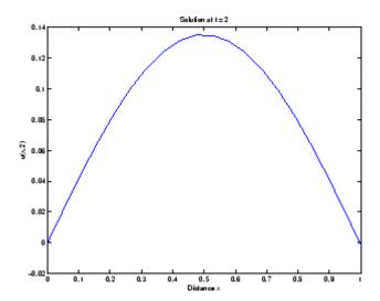
**Evaluating the Solution.** After obtaining and plotting the solution above, you might be interested in a solution profile for a particular value of t, or the time changes of the solution at a particular point x. The kth column u(:,k) (of the solution extracted in step 7) contains the time history of the solution at x(k). The jth row u(j,:) contains the solution profile at t(j).
