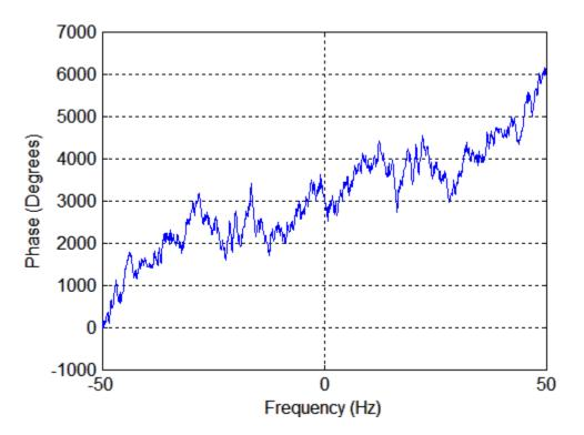
Component frequencies are mostly hidden by the randomness in phase at adjacent values. The upward trend in the plot is due to the unwrap function, which in this case adds  $2\pi$  to the phase more often than it subtracts it.
