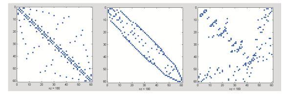
The reverse Cuthill-McKee ordering, r, reduces the bandwidth and concentrates all the nonzero elements near the diagonal. The approximate minimum degree ordering, m, produces a fractal-like structure with large blocks of zeros.
