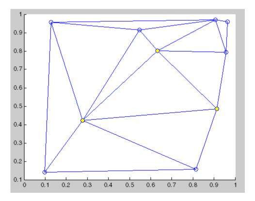
MATLAB classes on computational geometry enable you to instantiate a geometric representation object and make changes to the object without altering the initial dataset. You can remove the point from the triangulation without altering the original data.
